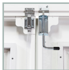
Standard doors have top and bottom cable operated lock latches to the active leaf and shoot bolts to the inactive leaf for dependable security.
